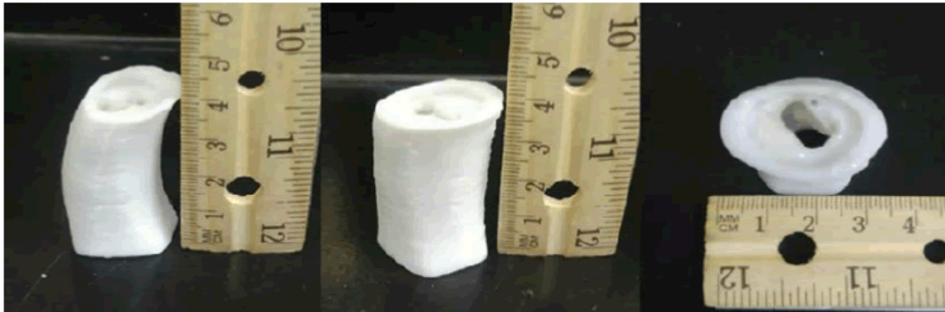
Figure 6 - PLA/PCL/TiO 2 Composites for Cancellous Bone
