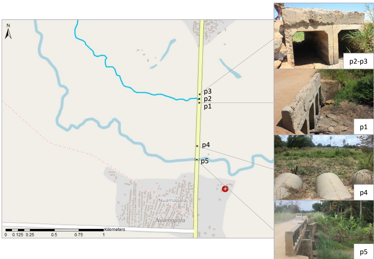
Figure 18 Outflow 1 detailed with photos
