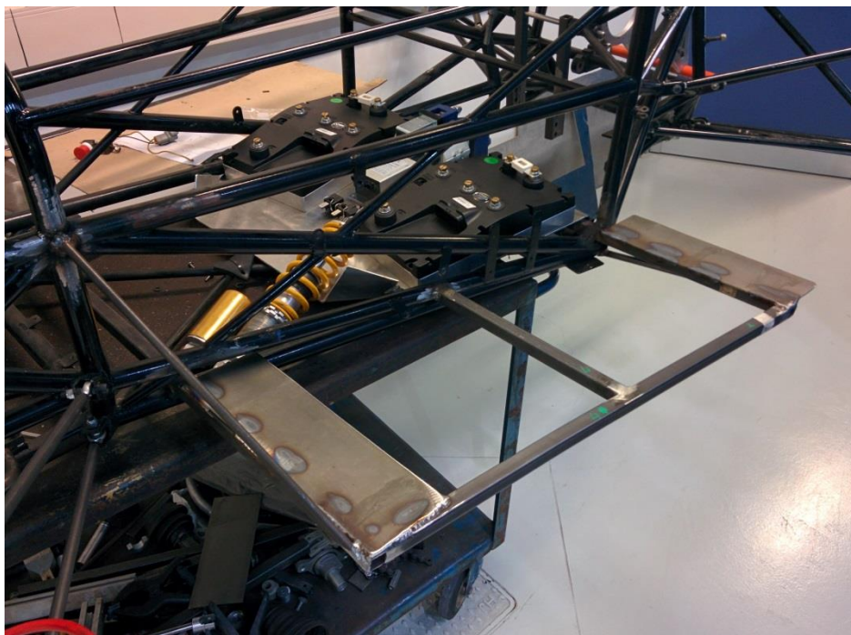
Figure 2-3. Battery brackets with steel plates
