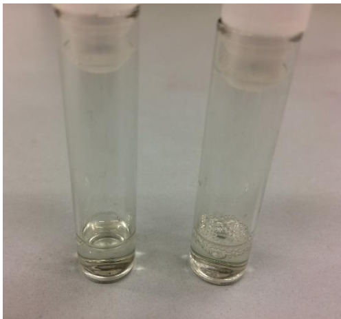
Figure 2.7 – BSA aqueous solutions (10% loading). On the left clear solution and on the right foaming of the solution.
