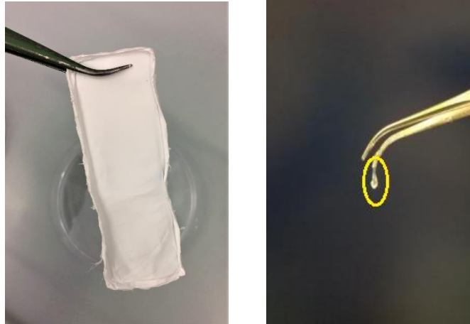
Figure 3.1 – A PVA/BSA mat (A) before and (B) after water interaction. An imminent severe shrinking was noticed.
