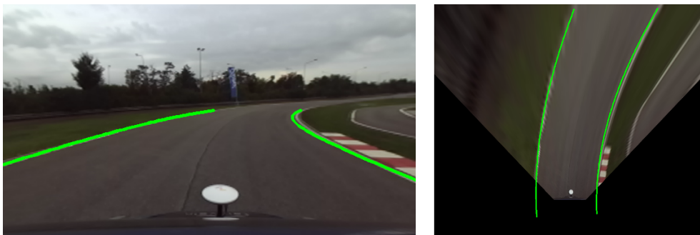
Figure 5.4: Line detection on an extensive road bend.
