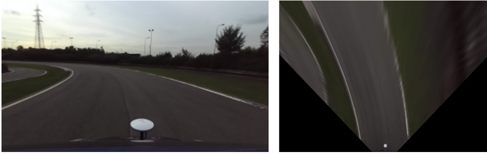
Figure 4.4: A front-view image acquired with our vehicle and the corresponding BEV representation.
