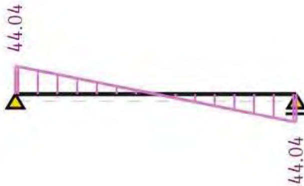
Diagram of the shear (S.L.S.)
