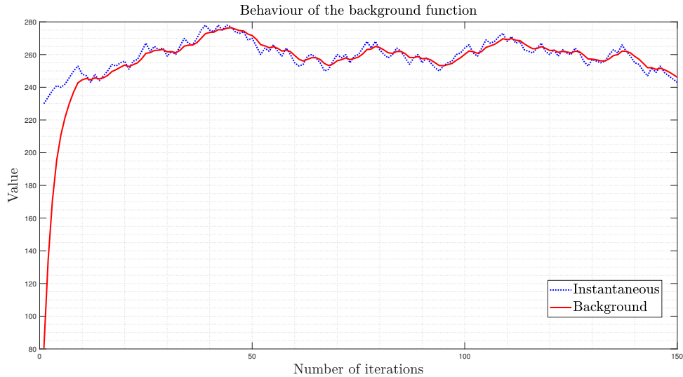
Figure 4.1: Background function response to random inputs. The dotted blue line shows the input data, while the solid red line the background function response. This simulation is performed over a single pixel.
