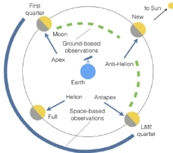
Figure 2.1: LUMIO science period. Solid blue line represent the period in which the S/C shall be in science mode. As can be seen this period coincides with the period without activity on Earth. Credits to: Topputo et al. (2017).
