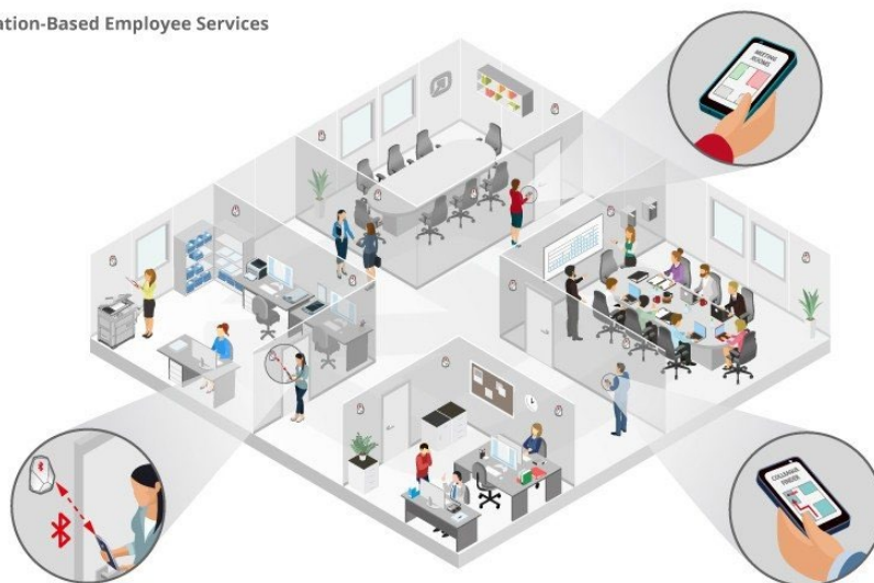
Figure 52 - The position is determined via a network of Bluetooth Low Energy (BLE) beacons. They emit signals which the app on the user's smartphone uses to calculate the position. The user is guided to his destination via turn-by-turn navigation. The "Colleague Finder" function enables sharing employees' position. (Source: Katja Streich, "Location-Based Employee Services", 23/02/2018)
