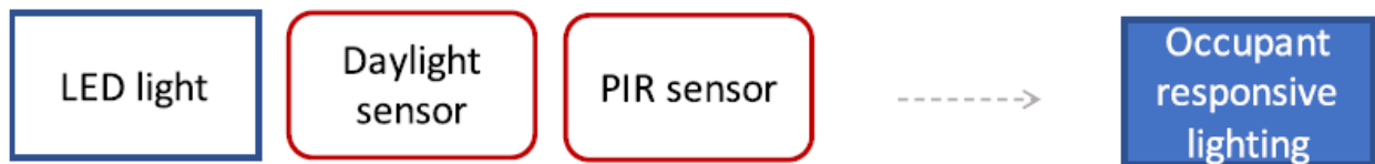
Figure 7 - Diagram of the functioning of an occupant responsive lighting. (Source: Ruoxi Jia, Baihong Jin, Ming Jin, Yuxun Zhou, Ioannis C. Kostantakopoulos, Han Zou, Joyce Kim, Dan Li, Weixi Gu, Reza Arghandeh, Pierluigi Nuozzo, Stefano Schiavon, Alberto L. Sangiovanni-Vicentelli, Costas J. Spanos, "Designing Automation for Smart Building Systems", 18/07/2018)
