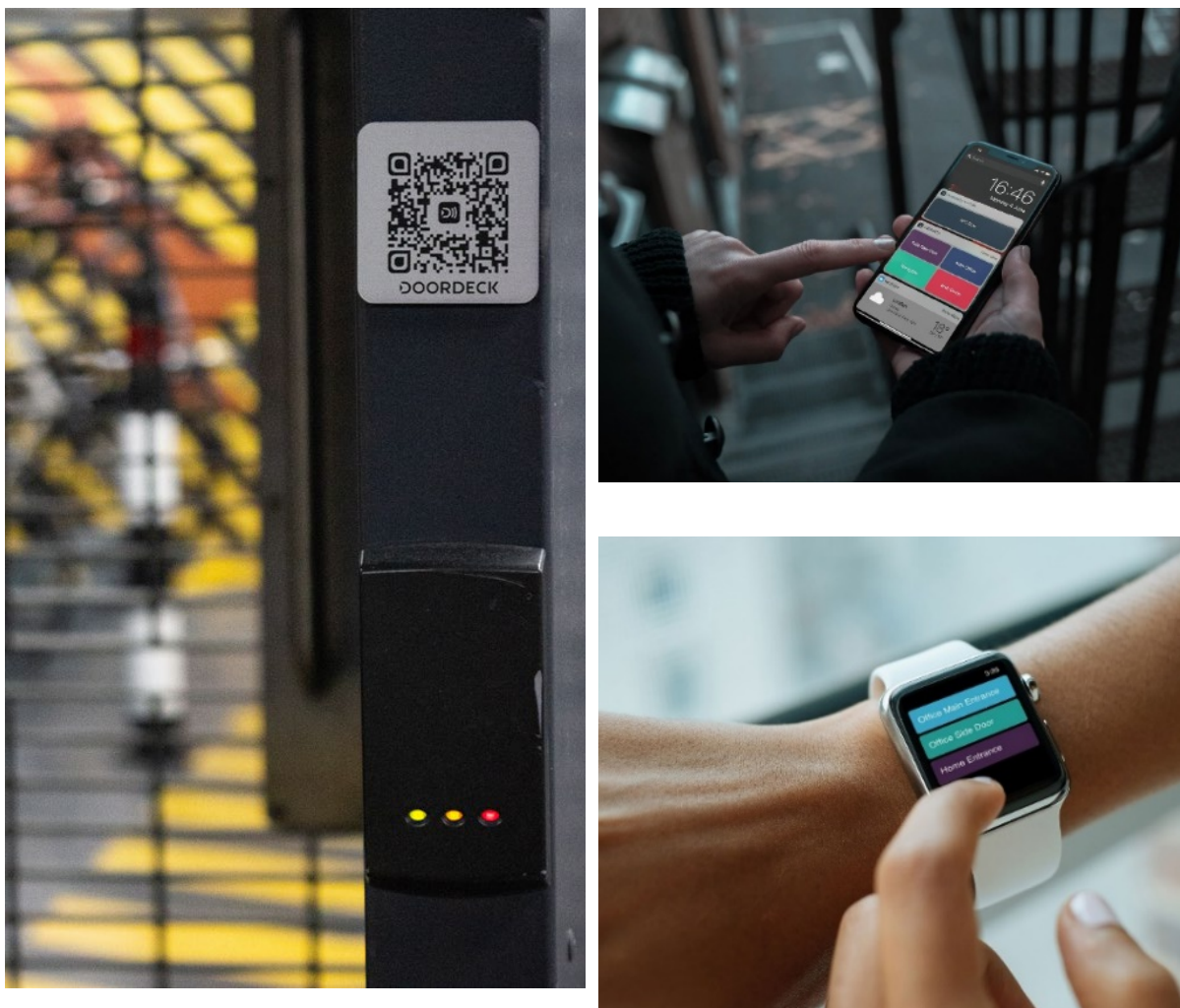
Figure 45 - The three images show how Doordeck system works: the QR code tile is installed on the door, and then it has to be selected on the smartphone or on the smartwatch that is the door to be opened (Source: Doordeck brochure).
