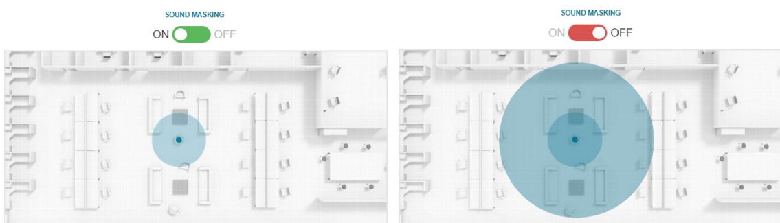
Figure 48 - The image on the left shows the radius of distraction when sound masking is on, and it is compared to the radius of distraction with sound masking off, which is considerably bigger, as the image on the right shows (Source: Cambridge Sound Management, "Sound Masking 101 technical brochure".)
