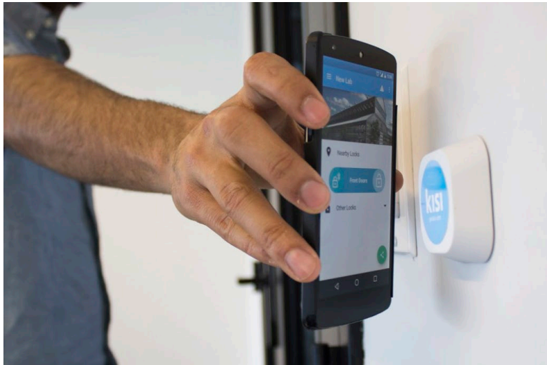
Figure 44 - Example of a keyless entrance method which uses an app installed on the smartphone to guarantee the access to the building (Source: https://www.getkisi.com/ ).
