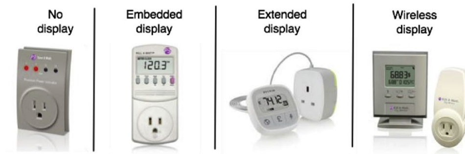
Figure 97 - Differences between load monitor hardware. (Source: Ford, et al. “Categories and functionality of smart home technology for energy management, 2017)
