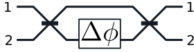
Figure 6.10: Schematic of a two port interferometric device. It is a well known Mach-Zehnder interferometer.
