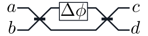
Figure 1.7: Mach-Zehnder interferometer schematic. The two input modes (a,b) are split and acquire a relative phase shift \Delta\phi before being recombined and output in modes (c,d).
