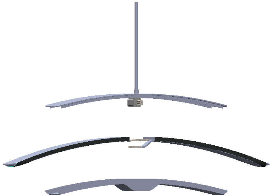
FIG 43. From up to bottom, Mechanical Input Subsystem Telescopic Arm Subsystem Main Shell Subsystem.
