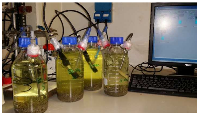
Figure 6.2: Microcosms Set UP and connection to MARTINA analyser.
