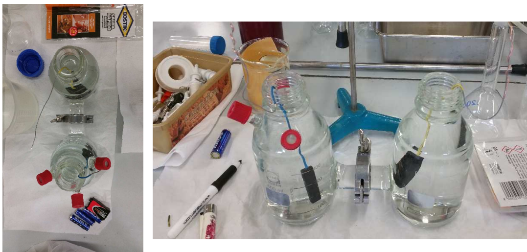
Figure 8.1. Dual-chamber H-shaped reactors (2C-MFC).
