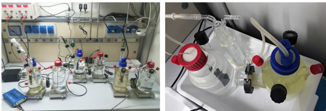
Figure 8.5. M3Cs, in thermostatic cell, at the end of the set-up phase.
