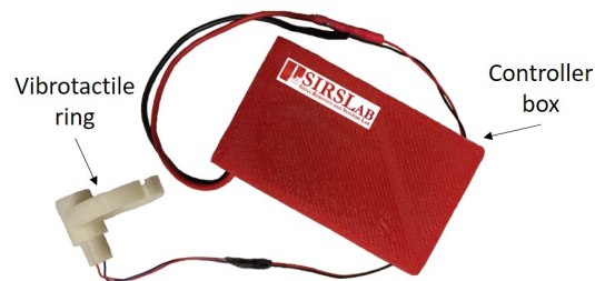
Figure 3.5: Vibrotactile ring with its controller box. During the experiments the ring is worn on the operator's left hand and the box is attached to a Velcro bracelet worn on the forearm.
