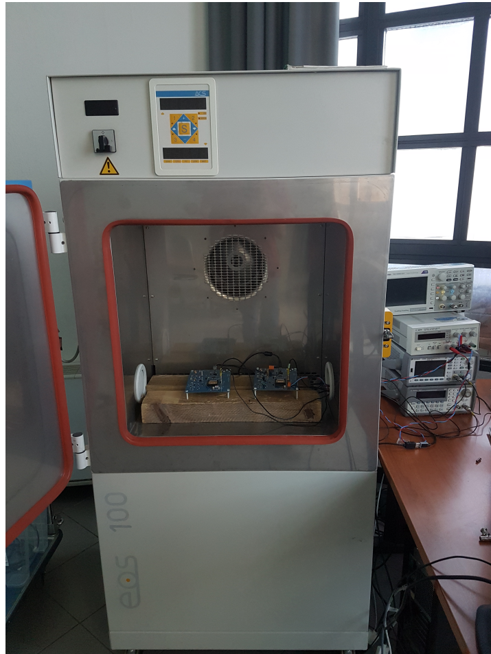
Figure 5.2: The board – in these case two identical boards to perform the measurements on two devices within the same temperature sweep – is placed inside a climatic chamber. The temperature was swept between 5 °C and 85 °C to avoid problems due to the condensation of water vapor inside the chamber. On the right it is possible to see the bench-top instruments used for the measurements.
