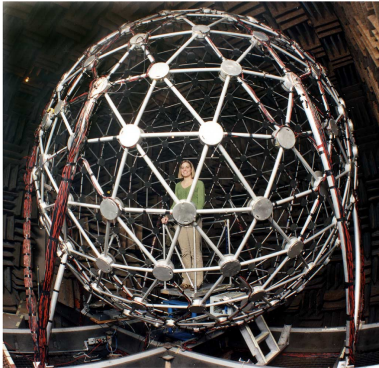
Figure 2.9: HRTF recordings setup at Auditory Localization Facility at Wright-Patterson AFB, Dayton, OH. Image taken from [4]
