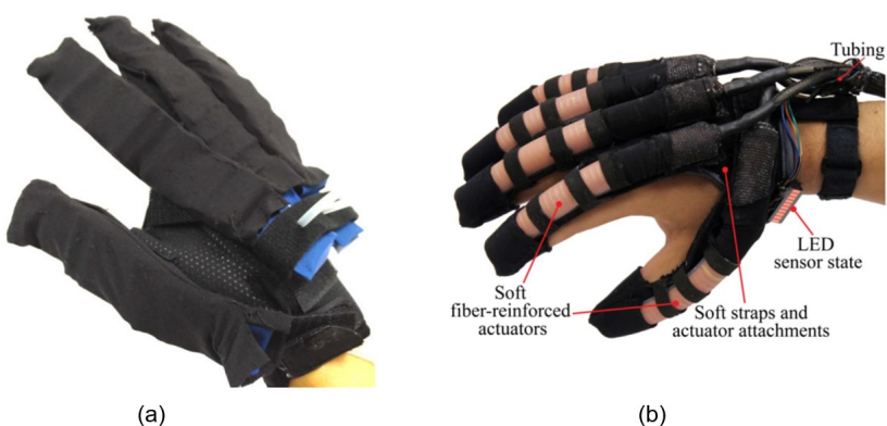
Figure 2.16: Exoskeletons based on soft-robotics: the Harvard Glove 2.0 [88] (a), and the NUS Glove [119] (b)
