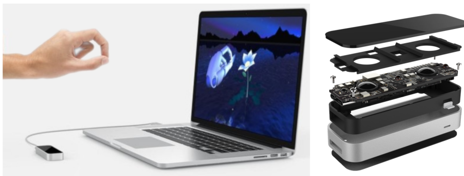
Figure 6.6: Principle and structure of the Leap Motion Controller [111]
