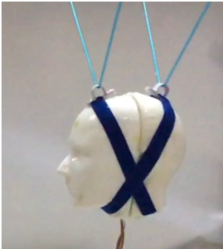
Figure B.6: The dummy head after assembling it with the Velcro straps [11].
