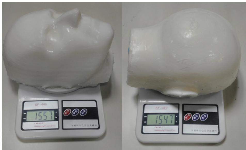
Figure B.4: The measured mass of the dummy head parts [11].
