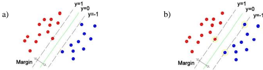
Fig. 7.3. Margin between two classes of data: a) general solution, b) maximization of the margin
