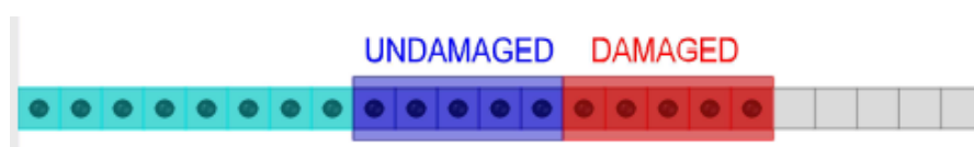
Fig. 7.6. Scheme of the first damage detection strategy (CSA, Consecutive Segments Analysis)
