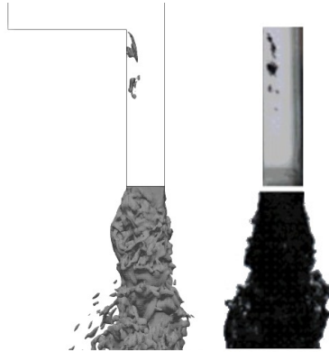
Figure 3.20: Internal nozzle flow test case [199]. Left) interPhaseChangeMixingFoam ; right) visualizations from experiments.
