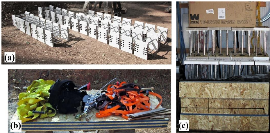
Figure 158. Disassembled (a) arch and (b) reinforcing materials, and (c) the stored system
