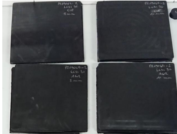
Fig. 2. 1. Four recycled rubber specimens under study.
