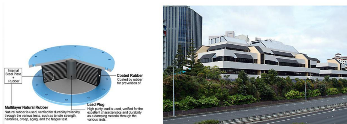
Fig. 1. 6. Detail of lead rubber bearings (LRB) (source: http://www.oiles.co.jp ), and the William Clayton Building in New Zealand isolated with LRB.
