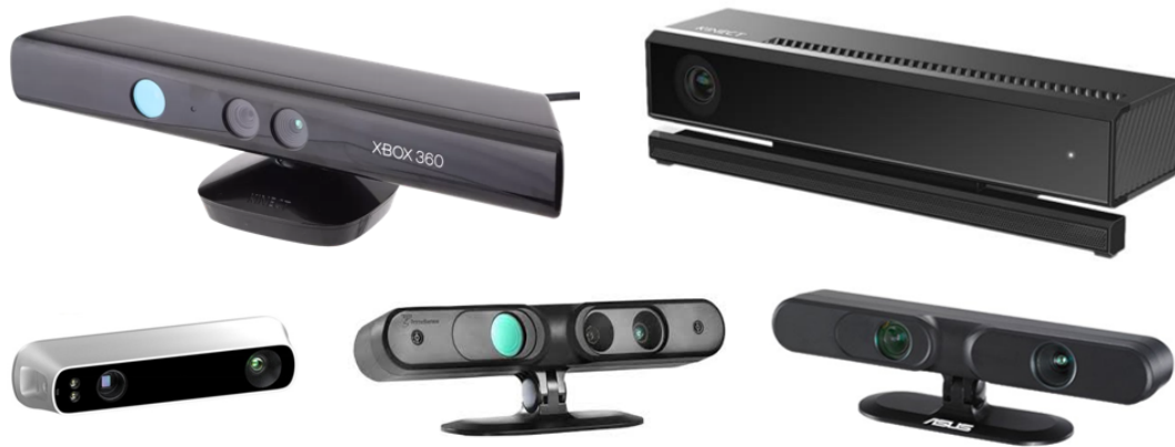
Figure 2.1: Low-cost devices used also for reverse engineering. Microsoft Kinect V1 and V2 in the top row, Structure Sensor, Prime Sense and Asus Xtion, in the lower row.
