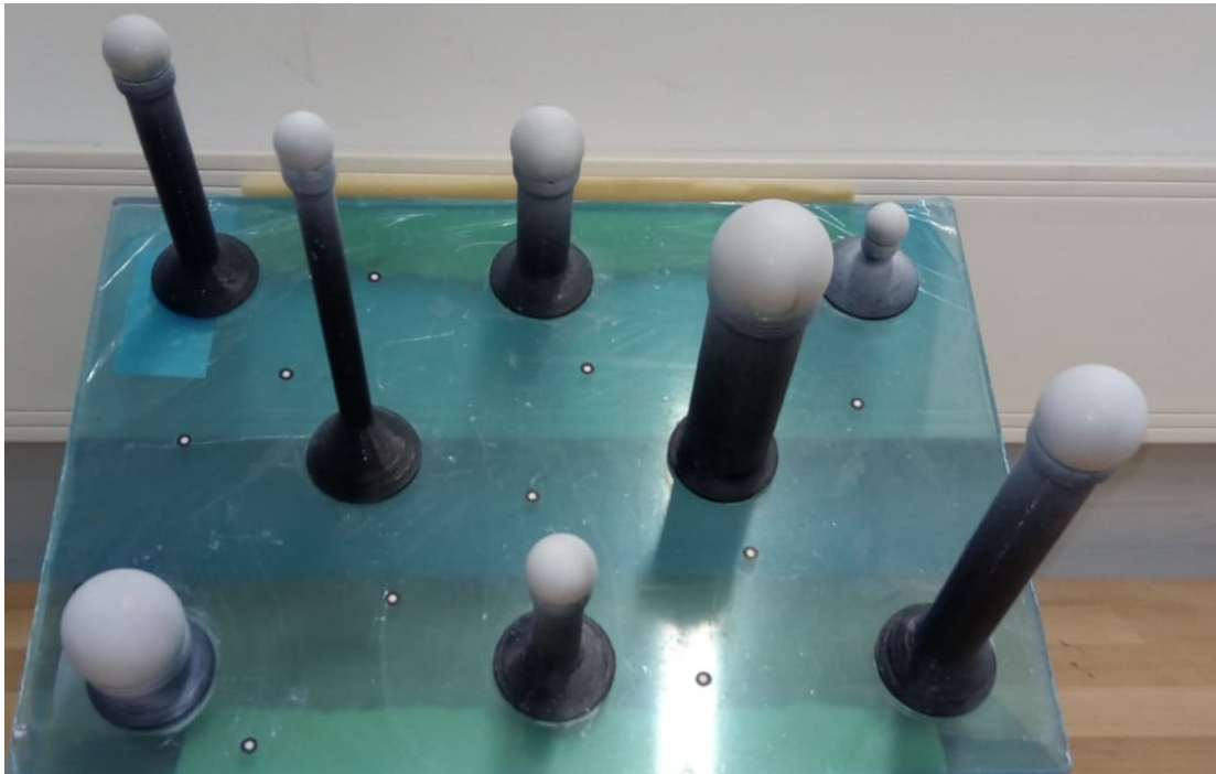
Figure 2.2: Sphere test object containing 8 spheres of different dimensions at different heights.
