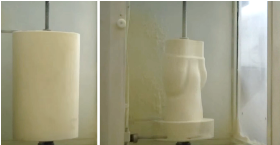
Figure 1.13: Initial polyurethane foam block (on the left) and lathing process in a CNC machine (on the right). In the lower part of the right picture it is possible to see the long drilling end-effector [7].
