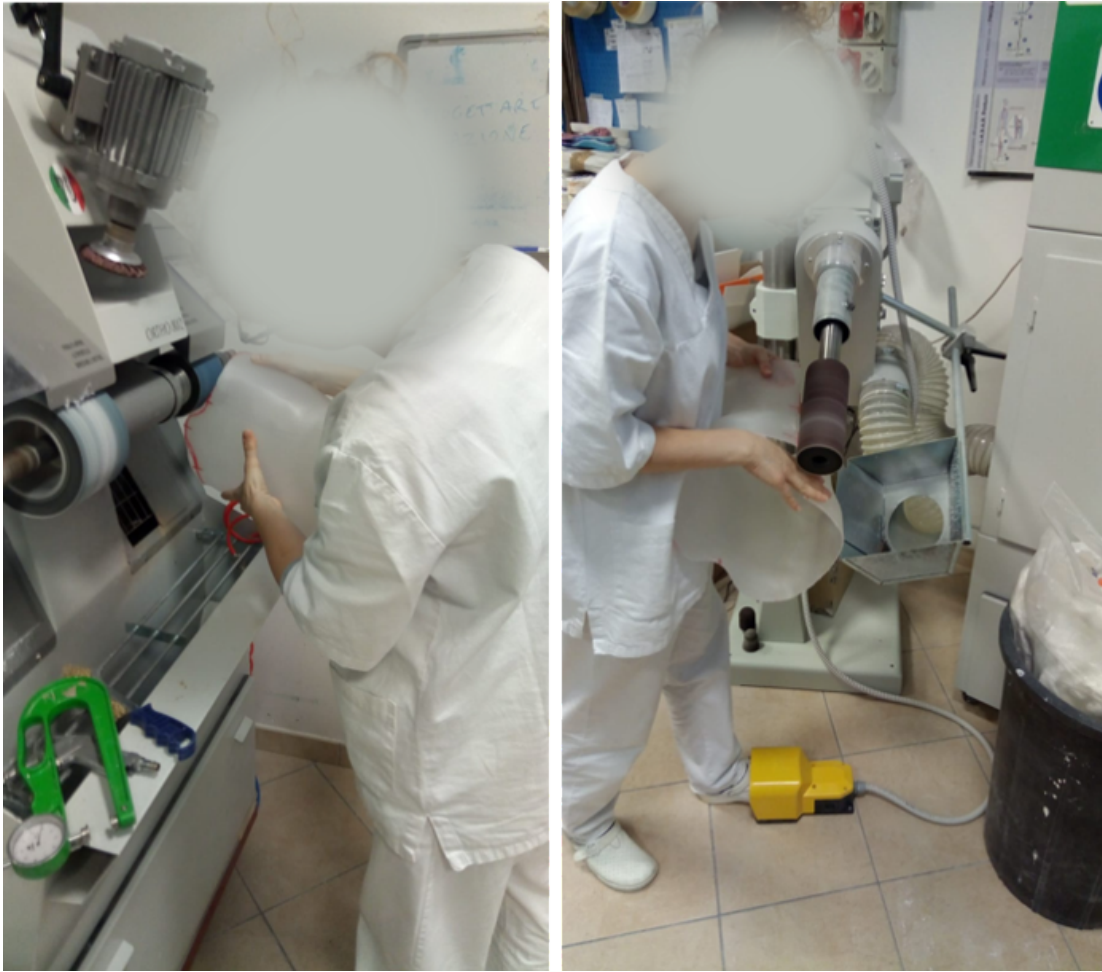
Figure 5.26: Manual post-processing of the 3D printed brace with rough and smooth grinders for the border.
