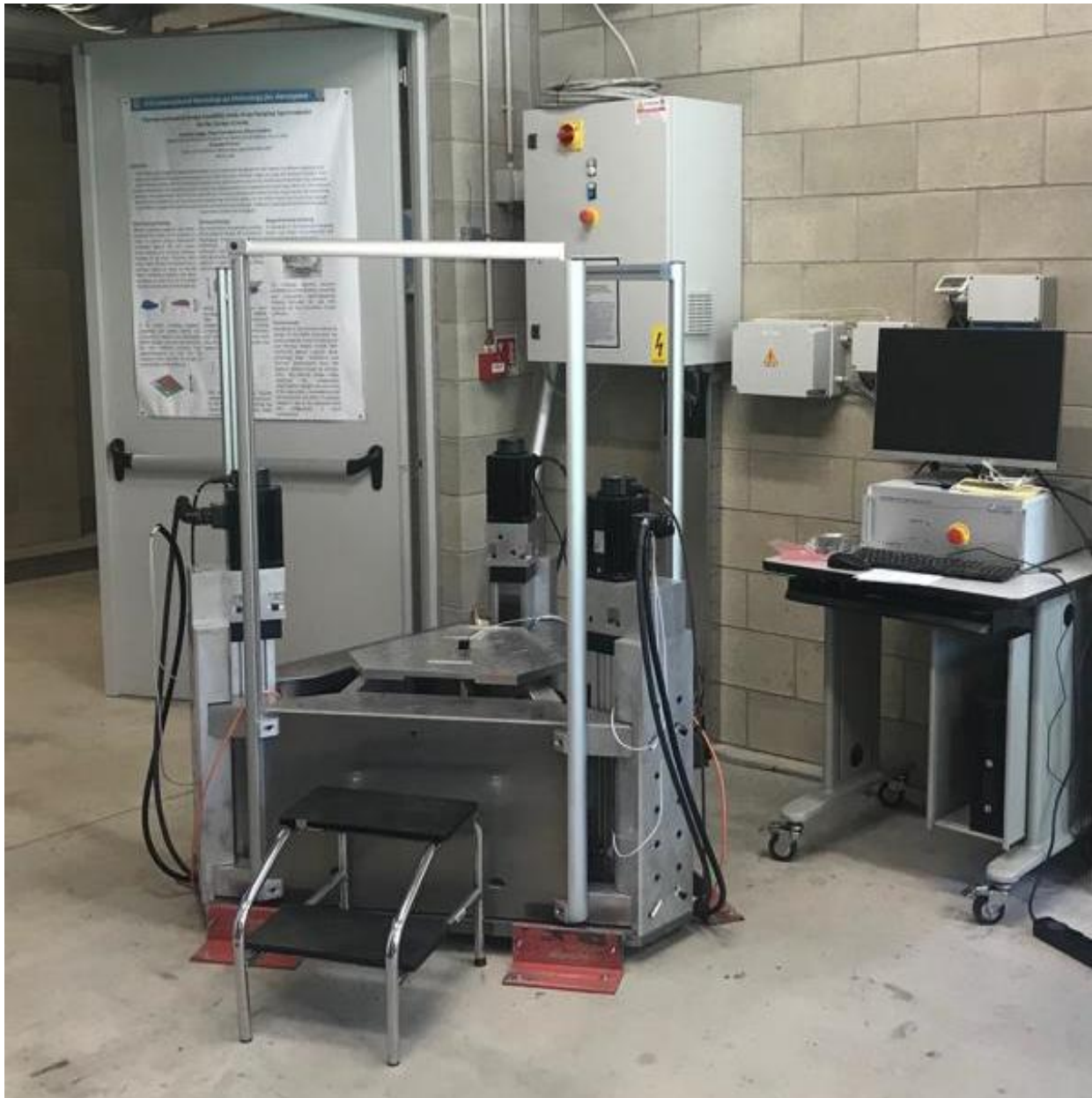
Figure 43: Picture of the Linear Delta Shaker inside the MetroSpace Lab, at Lecco campus of Politecnico di Milano
