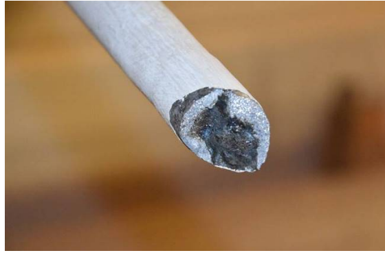
Figure 3- 13 Broken tie rod in August 2016 (Parisi et al. 2018)
