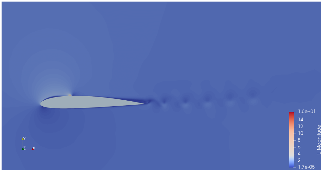
Figure 4.29: Contour velocity when f = 10 * \omega_n
