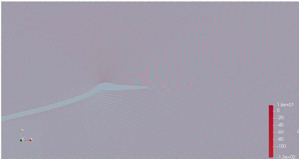
Figure 4.31: Streamlines with AFC - Constant Sucking
