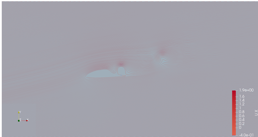
Figure 4.11: Streamlines without AFC
