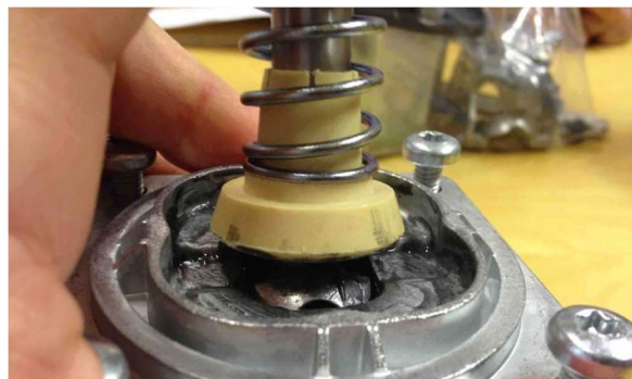
Figure 3.18: Spring in joystick
