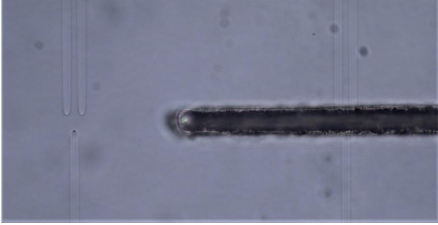
Figure 5.11: Microscope image of Structure 1 (left) and structure 2 (right) at the interface between the waveguides when the separation between the output waveguides is  $D = 15 \mu\text{m}$ .
