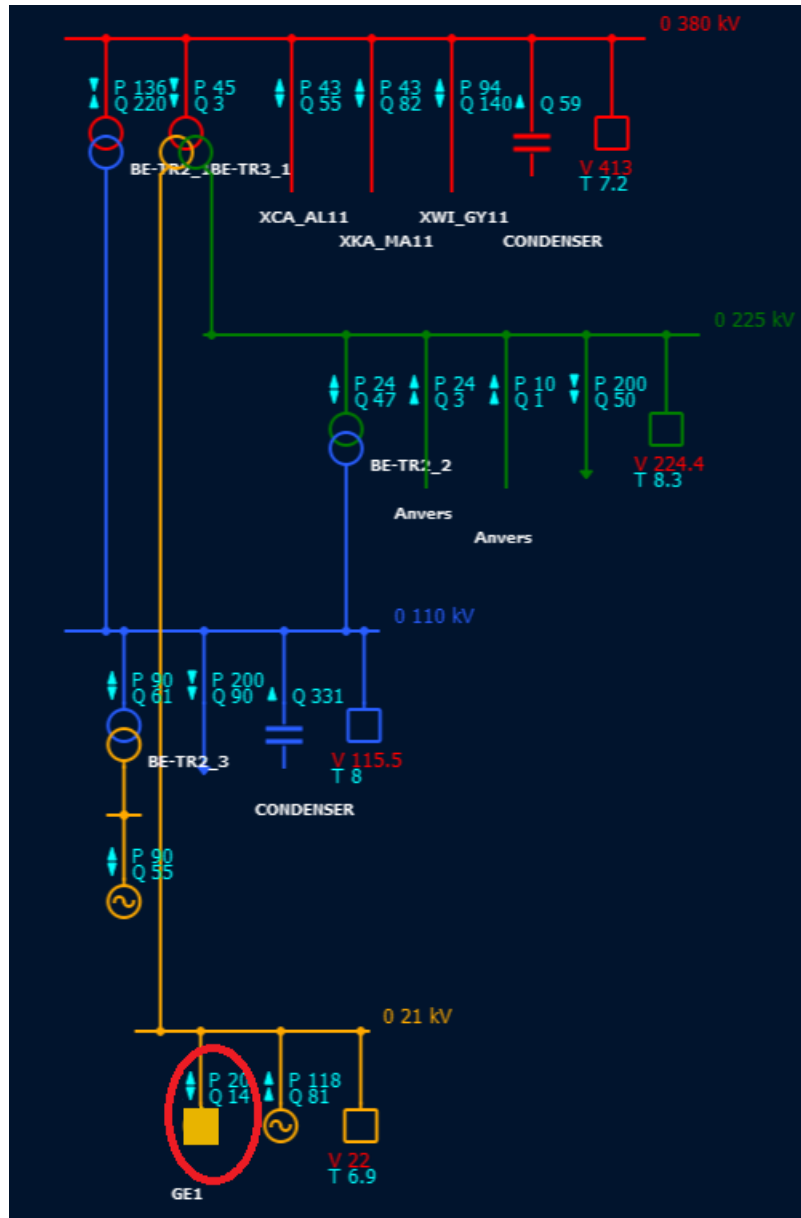
Figure 6.17- Illustration of the micro test network. The photovoltaic generator is highlighted by the circle in red.
