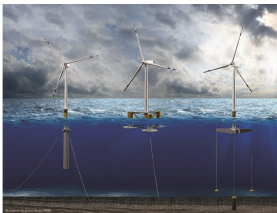
Figure 1.2: main floater types: spar buoy (left), semi-submersible (middle), and tension-leg platform (right). Source: Josh Bauer/NREL
