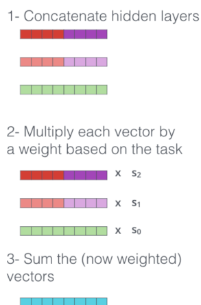
Figure 2.12: Steps to go from biLSTM hidden states to ELMo embeddings
