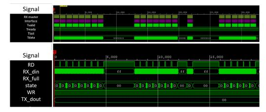
FIGURE 4.1: Waveforms when sending data to the FPGA without receiving.
