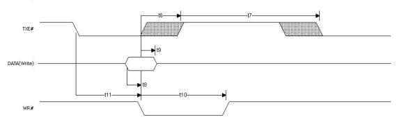
FIGURE 2.5: FT245 Asynchronous FIFO mode waveforms for writing [13].
