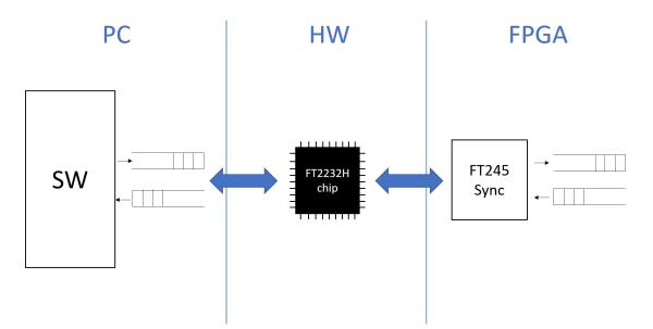
FIGURE 3.1: Structure of the data path.
