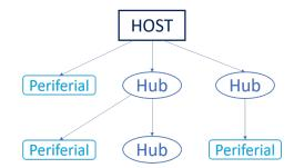
FIGURE 2.1: USB network structure.
