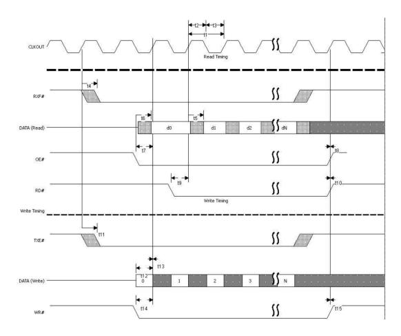
FIGURE 2.6: FT245 Synchronous FIFO mode waveforms [13].
