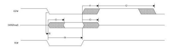
FIGURE 2.4: FT245 Asynchronous FIFO mode waveforms for reading [13].
