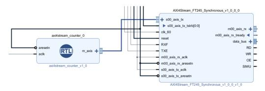
FIGURE 4.2: Block design to test the path FPGA-PC.
