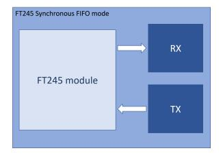
FIGURE 3.2: Block structure of the FT245 Synchronous FIFO interface.
