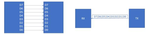
**FIGURE 1.2:** Parallel (left) vs serial communication (right).
