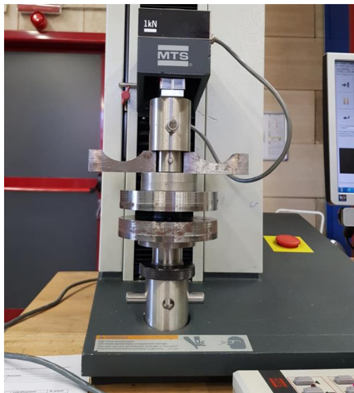
Figure 2.4: Sorbothane Pad under Compression test
