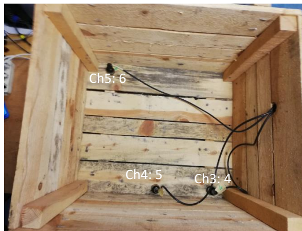
Figure 5.22: Accelerometer placed inside the crate - Ch 4 - Ch5 - Ch6 - PCB393B12
