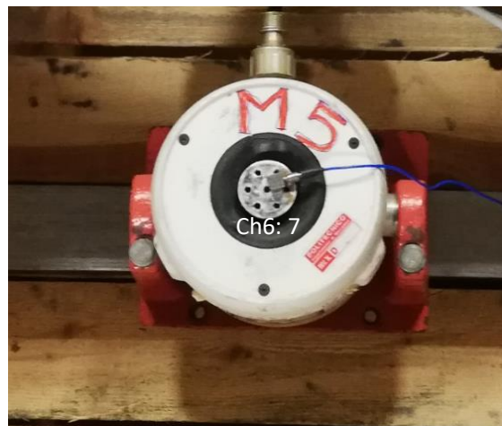
Figure 5.23: Accelerometer placed on the moving mass of the shaker - Reference - Ch6- PCB333B30
