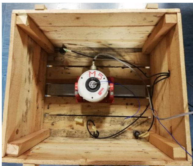
Figure 5.25: Configuration 1 - Shaker positioned over steel plate
