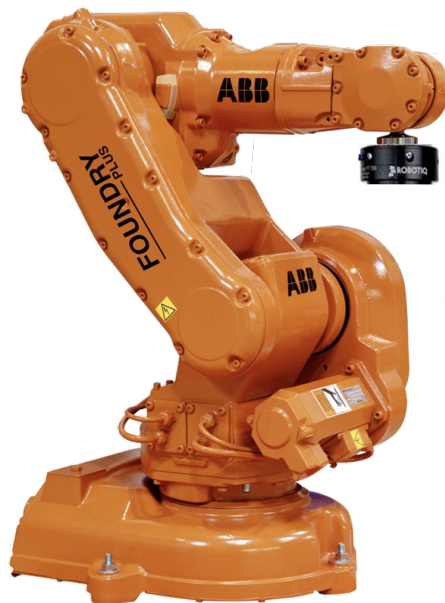
Figure 4.1: IRB 140 manipulator equipped with a 6 axis Robotiq FT300 F/T sensor
