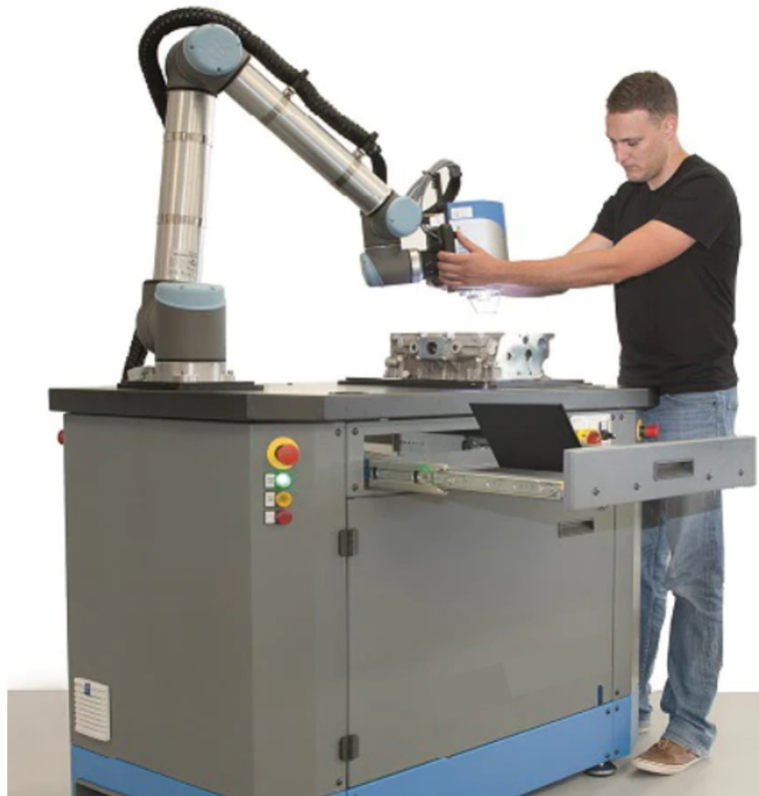
Figure 1.4: Quality inspection process using a collaborative robot physically interacting with the human operator
