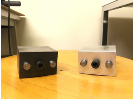
(a) Stages made from aluminium and steel
