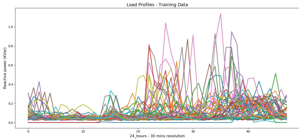
Figure 60. Reactive power profiles - second customer
