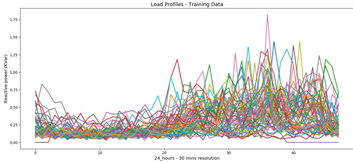
Figure 59. Reactive power profiles - first customer
