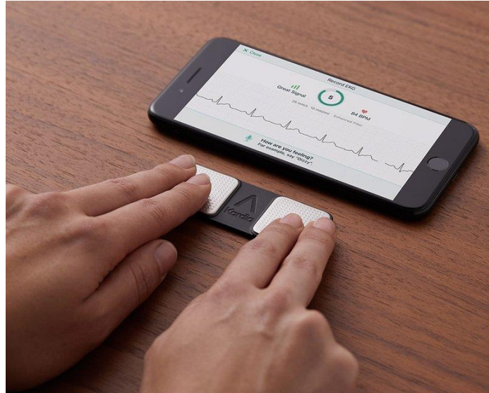
Figure 1.2.1 The Kardia Mobile App by AliveCor company transforms the smartphone in a standalone medical device for ECG and atrial fibrillation detection approved by the Food And Drug Administration (FDA). The results can be read by the user and also e-mailed to a physician. Image available on: https://www.alivecor.com/kardiamobile .
