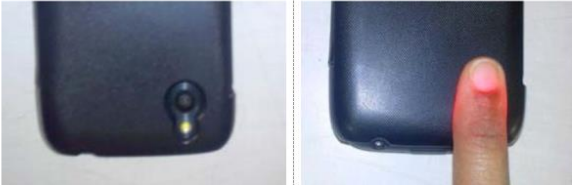
Figure 1.2.11 An HTC hero used reflection mode for PPG acquisition (Abinaya, Prabhakaran and Jaisankar, 2014).
