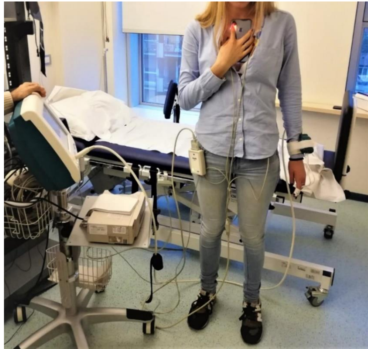
Figure 3.2.3 Configuration of Nexfin ECG module electrodes and the Nexfin cuff on the index finger of the left hand of the subject. The smartphone was positioned on the upper-middle chest.
