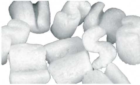
Figure 3.2: MEDEWO FILL-PAC Bio chips. The diameter of the chips were about 3 cm
