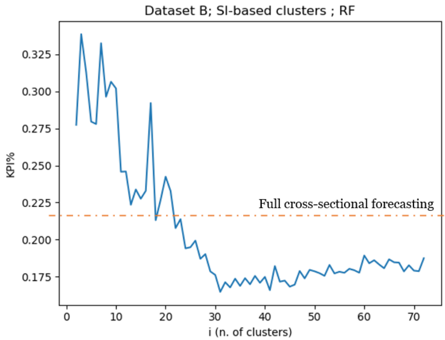
Figure 34: Average performance of RF on Dataset B as a function of the number of clusters formed used the SI-based clustering methodology
