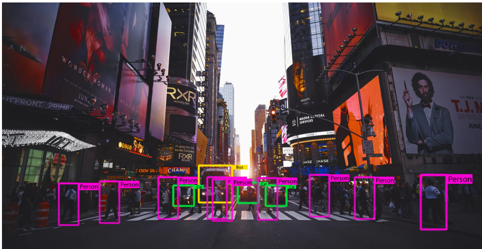
Figure 2.3: Results of an object detection system in action. Image created from a picture taken at [46]
