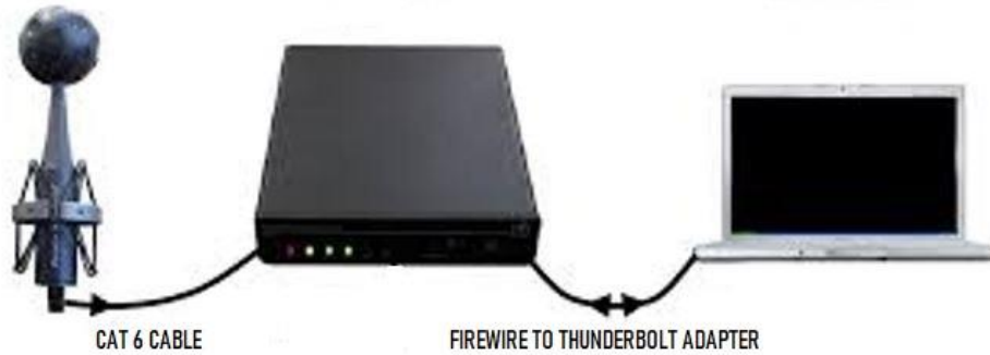
Figure 3: Eigenmike system setup
