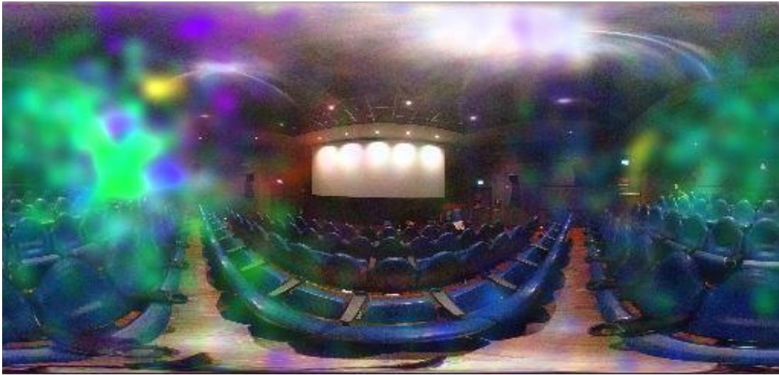
Figure 17: Cinema Lux sound distribution at 18 sec
