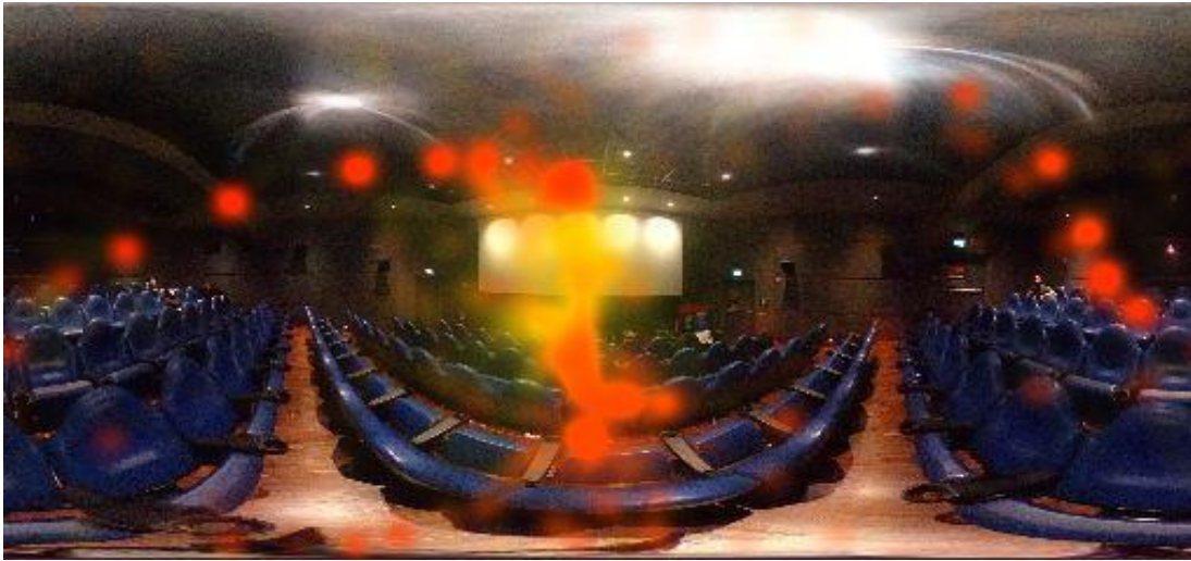
Figure 15: Cinema Lux sound distribution at 10 sec
