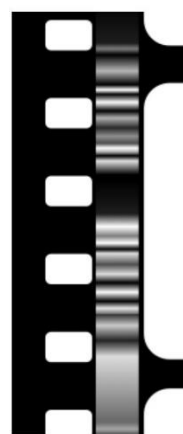
Figure 4: Variable density recording
