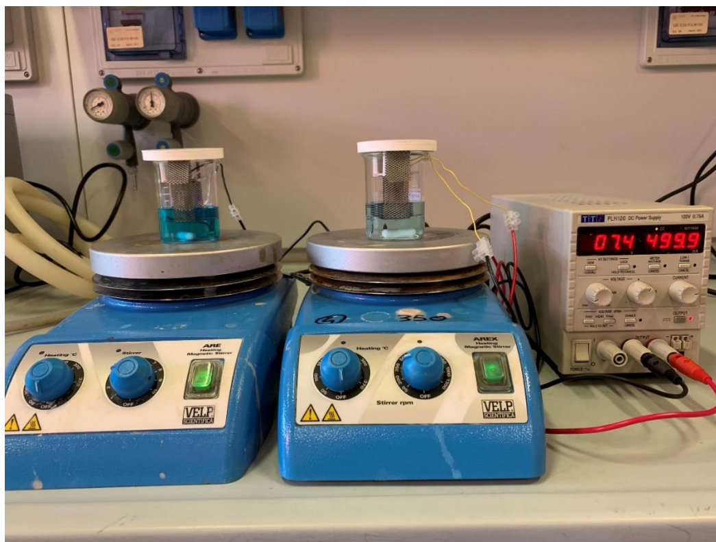
Figure 2.14. From left to right are presented 2 tests on methylene blue, the first one just started while the second has been going on for 3 hours.
