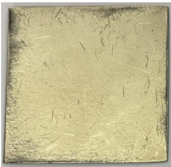
Figure 2.1. Titanium sample 3 cm x 3 cm pre-polishing.
