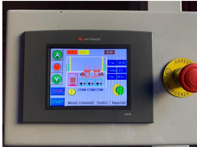
Figure 2.5. Control panel of the anodizing machine
