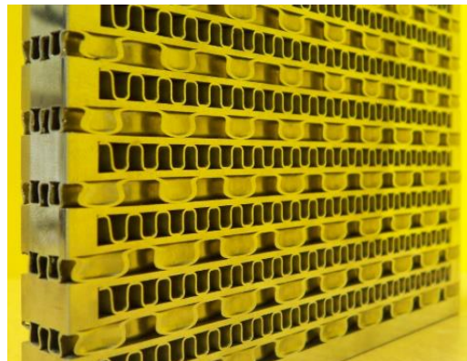
Figure 5.3 Section of a FPHE (cross-flow) [83]
