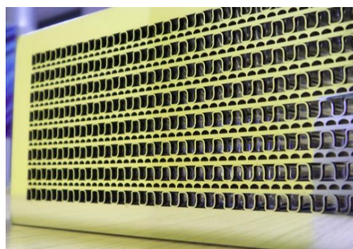
Figure 5.4 section of a H^2X (counter-flow) [83]
