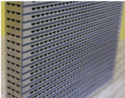
Figure 5.2 Section of a PCHE (cross-flow) [83]
