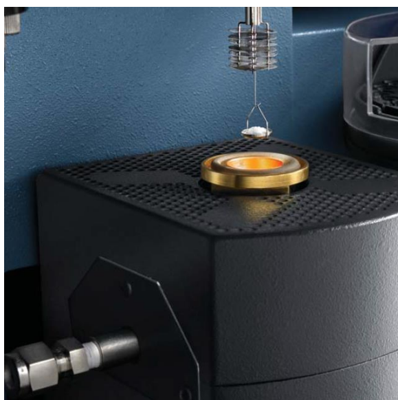
Figure 2.21 Furnace detail of TA Instruments TGA Q 500.
