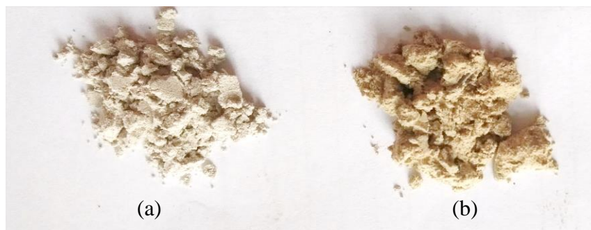
Figure 3.8 Picture of bioash from trial plant (a) and bioash from current plant (b).
