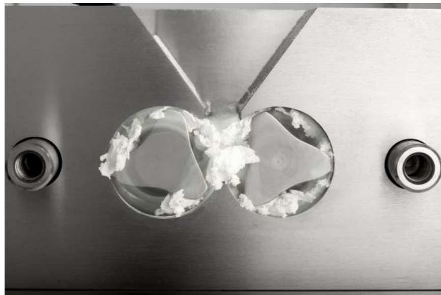
Figure 2.9 Brabender R - Lab Station 7 with Roller Mixer W50, detail of mixing camera.
