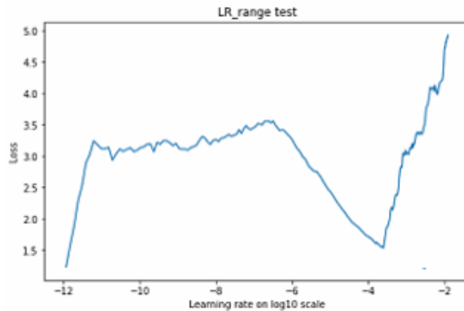
Figure 4.1 Learning rate test. Class-weighted loss function vs learning rate. At each batch update the learning rate is exponentially increased and corresponding loss function is reported. Good learning rates should be values from 10^{-6} and 10^{-4} , where the cost function decreases.
