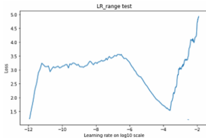
Figure 3.12 Example of learning rate range estimation. Class-weighted loss function vs learning rate in Log10 scale is plotted. The minimum learning rate at which the networks already learns is identified by the point in which the loss starts to fast decrease( 10^{-6} ). The maximum boundary is where loss starts to increase ( 10^{-4} ).
