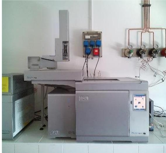
Figura 5: GC-FID Master GC- Fast gas chromatograph
