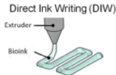
Figure 3.1 Representation of a DIW mechanism
