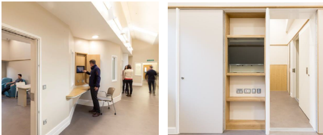
Figure 7.49 Electronic device are hidden in cabinet of corridor (Left) and inpatient's room (Right) (Source: Autism Inpatient Unit of Mitford Hospital)
