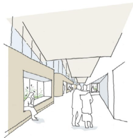
Figure 8.60 Window seat as transition space between inside and outside
