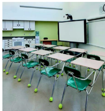
Figure 7.22 Additional sound absorbing ceiling hanging in waiting area (Left) (Source: Acoustic solutions for healthcare building designed by Ecophon) Figure 7.23 Chairs with tennis balls attached to the legs reduce noise (Right) (Source: Kristi Gaines, 2017. Design for autism spectrum disorder/p.74)
