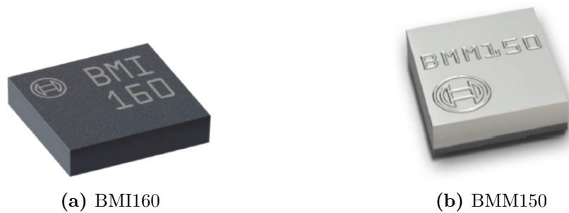
Figure 2.4: Bosch Sensortec BMI160 IMU with gyroscope and accelerometer and BMM150 magnetometer equipped on the Texas Instruments BOOSTXL Sensors BoosterPack plug-in module.
