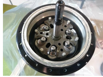
Figure 4.4: CVT rolling spheres along with their arms
