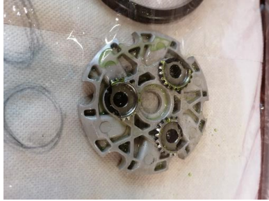
Figure 4.3: CVT gear change mechanism
