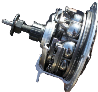
Figure 1.1: Sectioned CVT transmission.[7]
