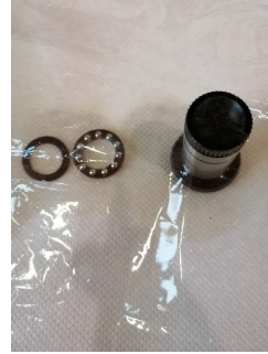
Figure 4.6: The CVT freewheel
