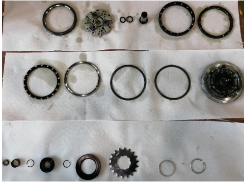
Figure 4.5: The components of the CVT from one side
