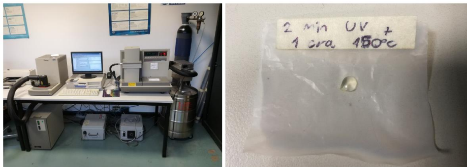
Figure 2.3: Left; DSC test platform Polimi Right: adhesive sample of the test
