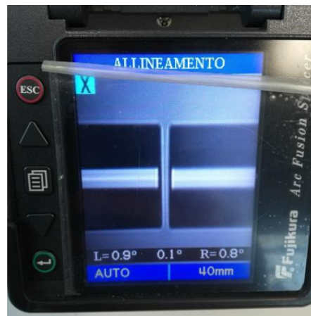
Figure 2.9: Correct alignment of the fiber
