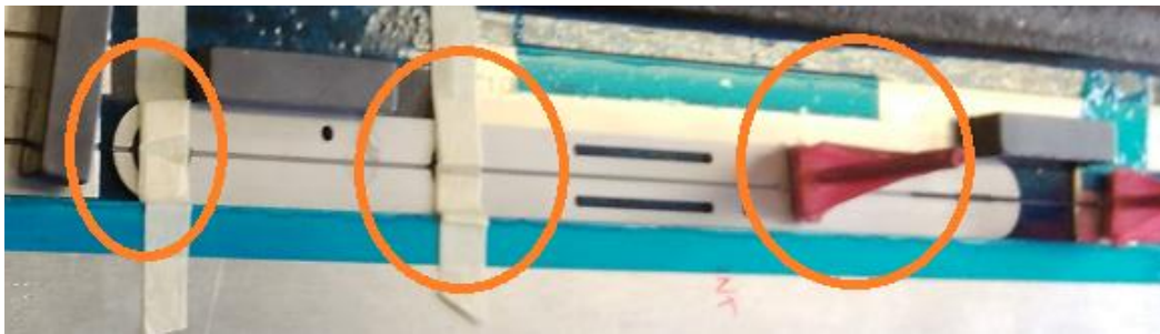
Figure 2.17: Ensuring the FBG sensor inside of the V-groove by mechanical means
