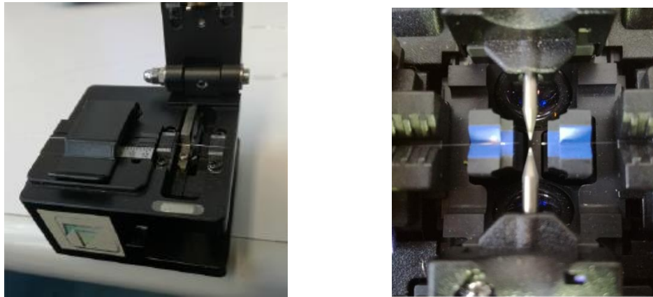
Figure 2.8: Splicer; FO junction tool Right; automatic positioning of the fiber
