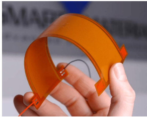
Figure 1.6: Smart Materials example; Macro fiber Composite actuator
