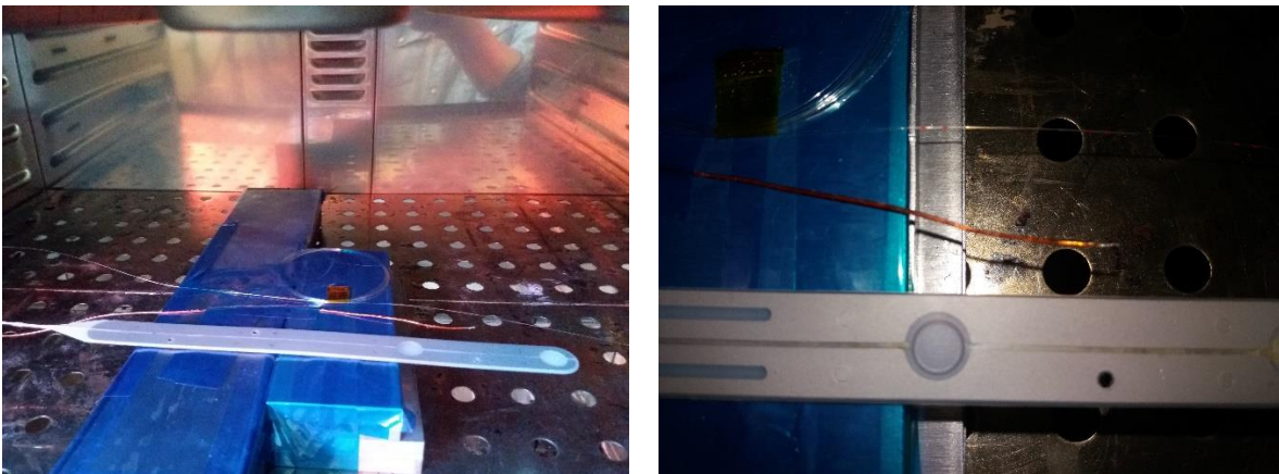
Figure 3.7: Three temperature measurements inside the oven
