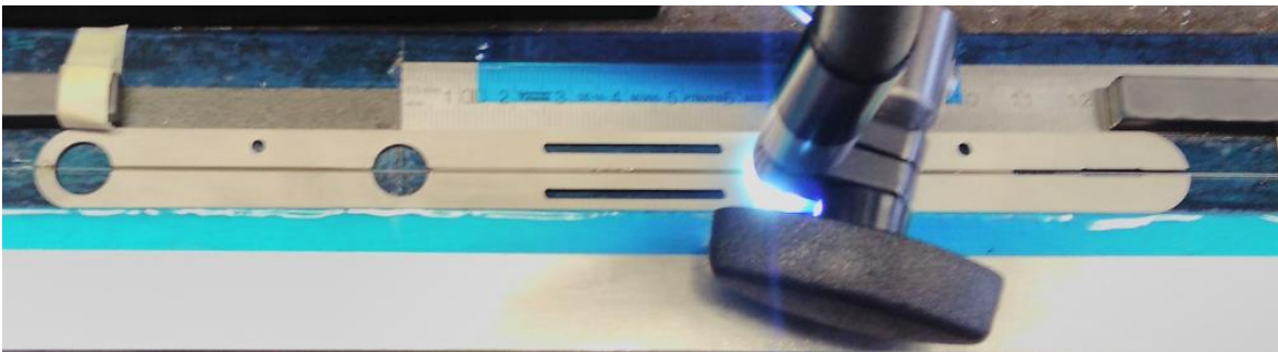
Figure 2.4: UV exposure curing cycle to SR in Polimi laboratory
