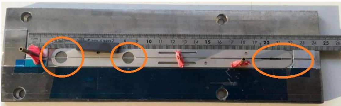
Figure 2.16: Correct positioning of fiber with metallic guides in the end and beginning of the fiber in circles
