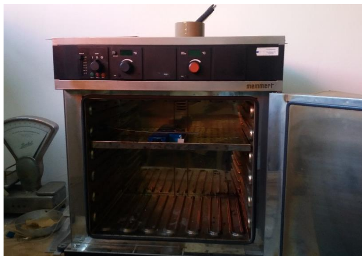
Figure 2.20: Final crosslinking of the adhesive in the oven
