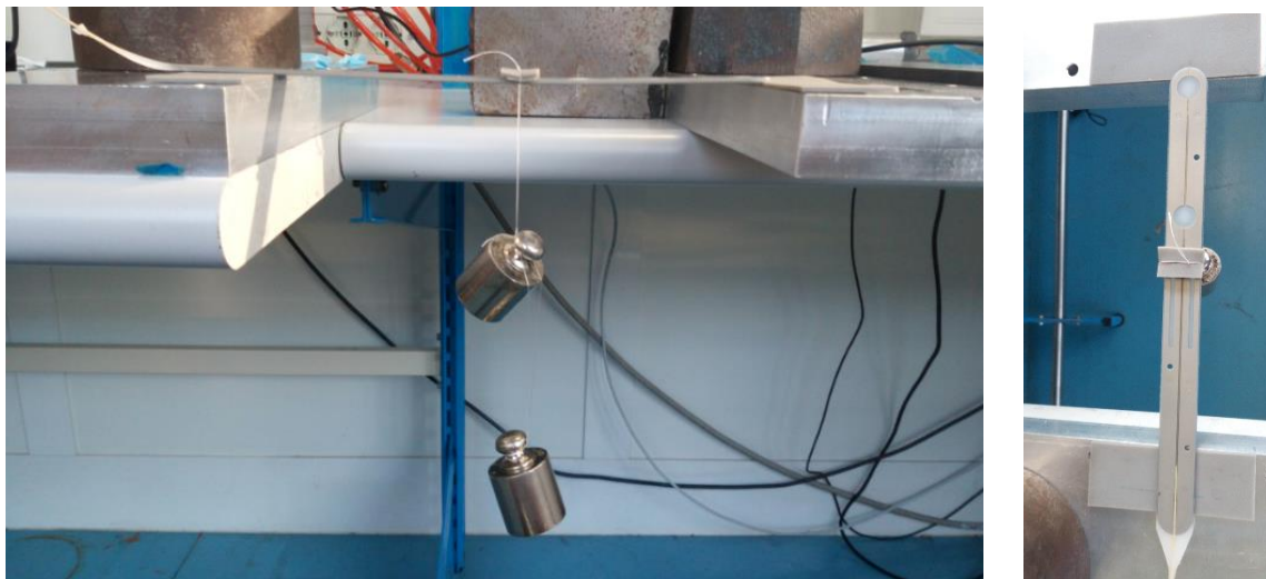
Figure 4.12: Flexural test in simple supported retractor
