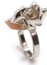
3D printed ring using SLA printed molds by "Anna Reikher"
