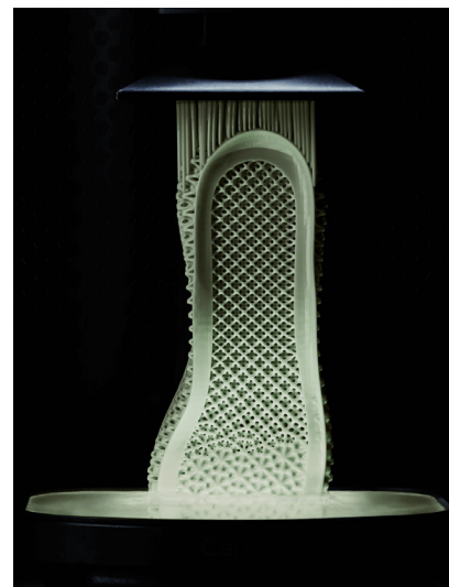
Adidas Futurecraft 4D sole's printing process in DLS
